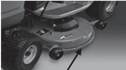
Armor Protected Stamped Deck Shell Example Below
